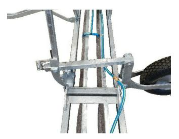
6.2m Wiper Main Frame Wheel & Extension Fitting
